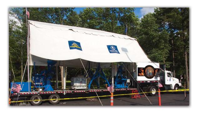
The Verdin Company designed and fabricated the world's only mobile foundry so that a bell can be cast on your site in full view of the public.
