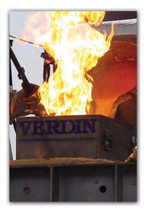
Once the furnace reaches 2,200 degrees, the molten bronze is poured into a custom bell mold, made especially for a customer, where it will cool and harden overnight. The bell must be cast in one continuous pour.
